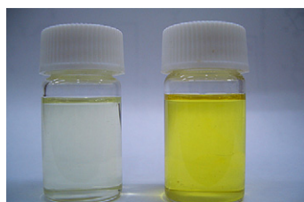
Figure 1. The photochromic switch of 23 and the color difference prior to and after photoirradiation ( \lambda=354 nm).
